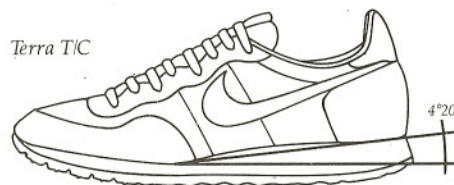
The Air-Sole® (top) in the Columbia, Aurora and Tailwind has different air pressure in the various sizes to give more appropriate cushioning. The Terra T/C (below) has a Pylon™ midsole also scaled for cushion as well as the same degree of heel lift in all sizes.
